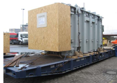
Cargo securing performed at the port terminal on a roll trailer
