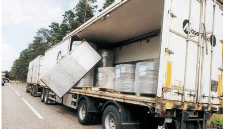
Trailer that has lost some of its load of pallets in the second layer.
