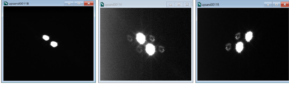
Figure 3. Defocused CCD images of images of \nu And in the B = 4400Å(left), V = 5500Å(center) and R = 7000Å(right) passbands. The faint "stars" visible on the V and R images are the reflections produced by dichroic beam splitters. They appear bright due to exaggerated contrast. In fact, the total intensity of reflection is < 0.1\% of that produced by stellar image.
