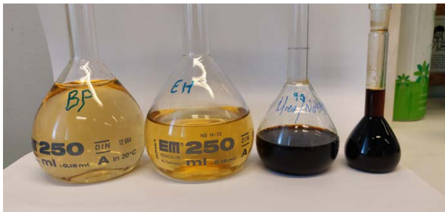
Figure 1. Lignin dissolution from left to right. BP in NaOH/water system; EH in NaOH/water system; BP in NaOH/urea/water system; and BP in ethylene glycol.
