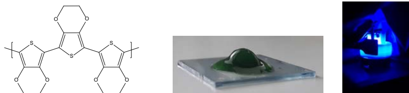
Picture 1. On the left: Structure of PEDOT. In the middle: Hybrid material after electrochemical measurements. On the right: Electrochemical measurements with blue light.
