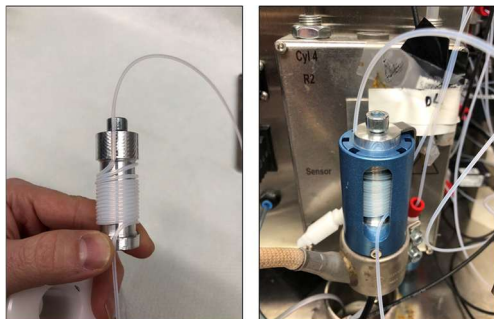
Figure 1. Simple flow reactor, at left, and the reactor fitted into the heating mantle of a radiosynthesis device.
