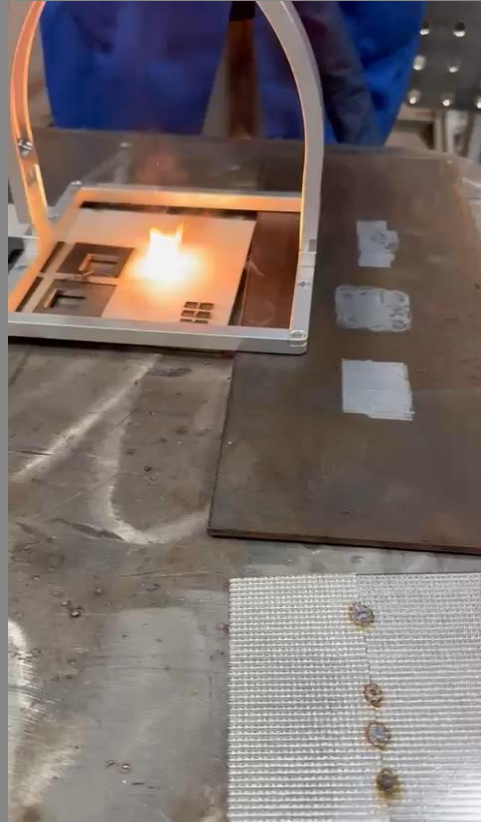
Cleaning of the coated maritime EH 36 steel sample
