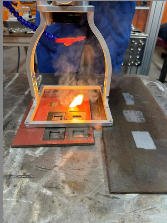
Cleaning of the thickest coated EH 36 maritime steel sample
