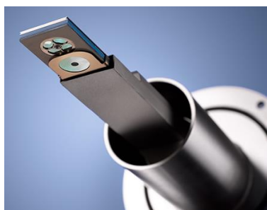
FlatQUAD detector with four chips for separate signal processing. Primary electron beam passes through the center hole. Image : www.bruker.com .
