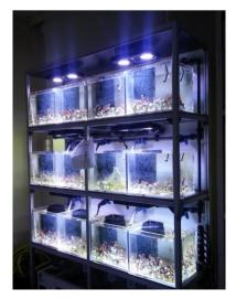
• **Filtration:** Our system boasts advanced filtration capabilities to maintain water quality. Seawater is pumped from a large head tank (approximately 200 liters) situated at the base of each rack to the individual aquaria, where it is then returned to the head tank. The water undergoes multiple filtration stages, including an acrylic filtration unit (SCHURAN Jetskim 120) equipped with both mechanical and biological filters, a protein skimmer, and UV radiation treatment.
